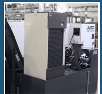
COOLANT REFRIGERANT CHILLER Upgrade from heat exchanger for precise temperature control regardless of ambient temperature.
