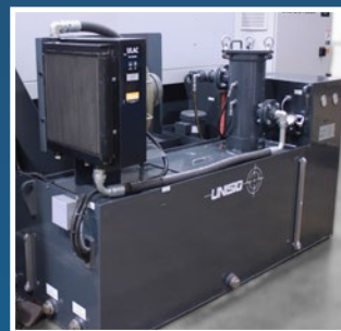
COOLANT HEAT EXCHANGER Remove heat from process and improve tool life, accuracy, and reduce mist.
