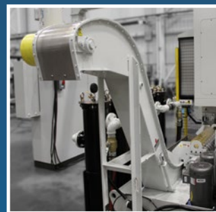
MAGNETIC CONVEYOR Upgrade from hinged belt conveyor for more efficient removal of chips.
