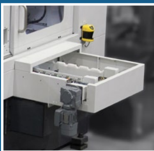
AUTOMATIC CONVEYOR LOADER Reduces labor and systemizes production.
