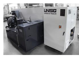
For added manufacturing flexibility, the UNE Series is small enough to fit almost anywhere, conserving valuable floor space. Its compact and stiff design eliminates the need for foundation work for effortless installation or relocation.
