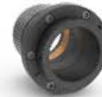
**Pressure heads** locate the workpiece, guide the drill, and introduce cutting fluid to the operation. The pressure head is a critical component in an accurate BTA process.
