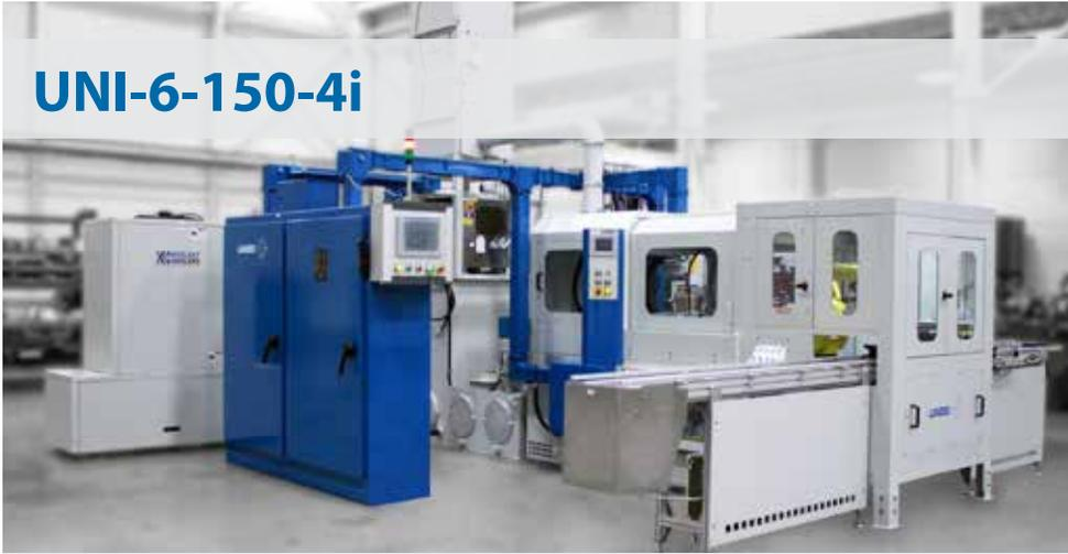
High-accuracy gundrilling of small parts with multiple off-center and angled holes from 0.8 mm to 6 mm [0.03 to 0.25 inch] diameter up to 150 mm [6.0 inch] deep.
