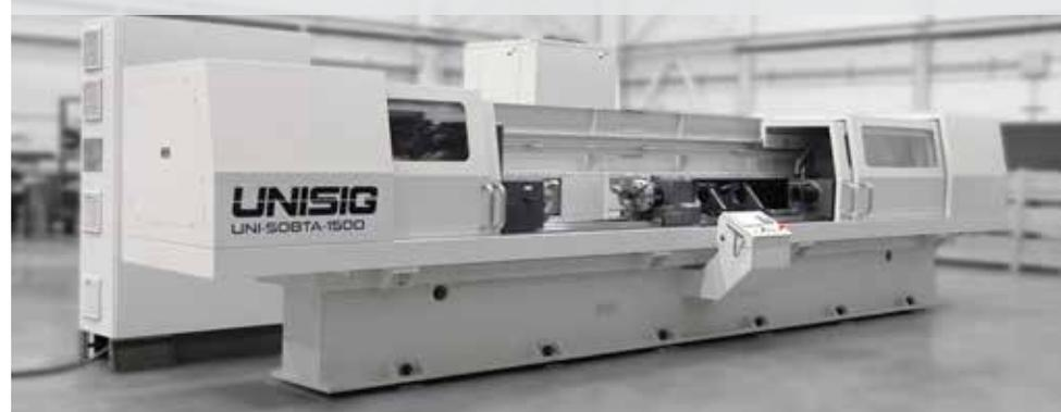
Versatile, high-precision machine for centerline bores up to 65mm [2.6 inch] dia and 1,500 mm [60 inch] deep in the toughest materials using gundrill and BTA tooling.
