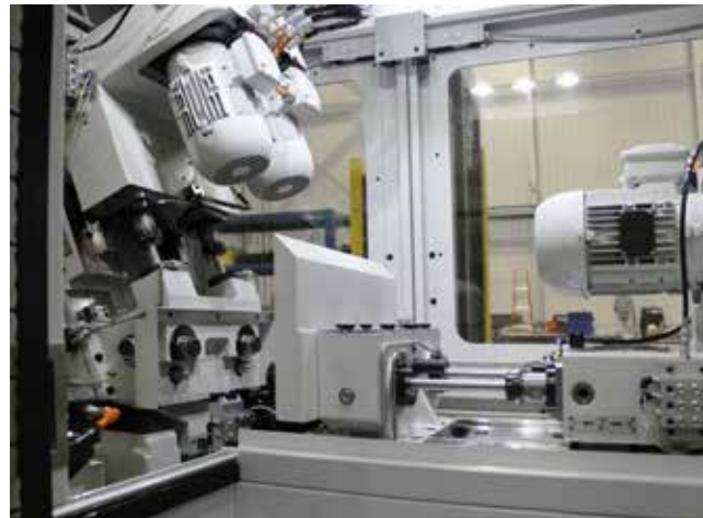
UNISIG UNI-Series automated machine for high volume production cell to manufacture power train components
