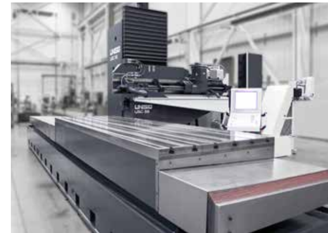
UNISIG USC BTA drilling machine with 50-taper milling spindle and special capacity table
