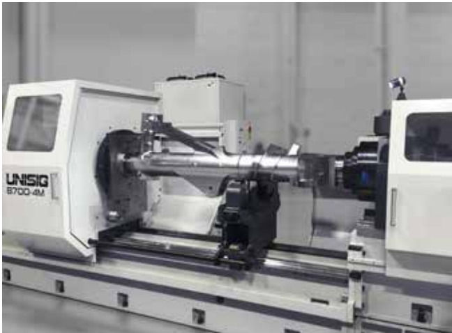
UNISIG B700 BTA machine with drop bed to swing up to 63 in [1600 mm] for commercial landing gear
